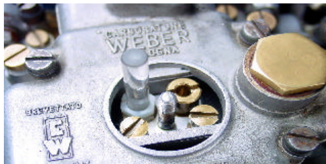
Figure 2: Using the Optical Gauge to Measure the Fuel Level
